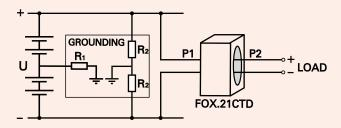
If the battery is not grounded at the centre point grounding resistors are required. Use either solution R1 if possible or the solution with 2 x R2.
