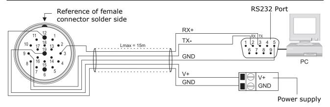
For RS232 connection, TX-, RX+ and serial GND signals (pin 9, 3 and 8 of M23 connector) are used, to be connected respectively to RX, TX and GND signals of RS232 port on PC (pin 2, 3 and 5 of 9-pole SubD connector). The length of RS232 cables should not exceed 15 m.
