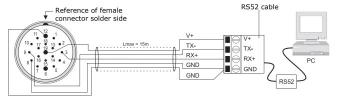
To use the **RS52** cable, the drivers included in the HD52.3D-S software package should be installed in the PC (see the guide to USB drivers installation included in the software package).
