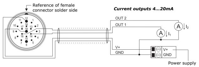
Current outputs are active. Load resistance: RL < 300  $\Omega$ .
