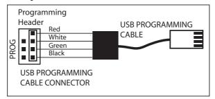
The correct process for connecting the controller via the USB is as follows:-
