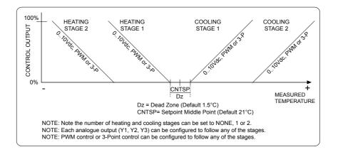
Between heating and cooling stage 1 is a control deadband. This prevent rapid switching between heating and cooling. The deadband is adjustable in the configuration parameters.
