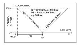
the setpoint the loop output is 100%. In the Direct Control mode the output modulates in reverse. The configuration is done via the configuration parameters (or over BACnet network).
