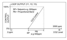
Proportional Band above the setpoint the loop output is 100%. The configuration is done via the configuration parameters (or over the BACnet network). The CO2 control loop can also be configured to operate as Proportional + Integral control by changing the Integral Action Time from 0 to a required value.
