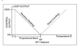
modulate to 100%. When the temperature is the amount of the Proportional Band below the setpoint the loop output is 100%. In the Direct Control mode the output modulates in reverse. The configuration is done via the configuration parameters using Device Configuration Tool or over the BACnet network.
