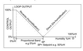
starts to modulate to 100%. When the humidity is the amount of the Proportional Band below the setpoint the loop output is 100%. In the Direct Control mode the output modulates in reverse. The configuration is done via the configuration parameters (or over the BACnet network).
