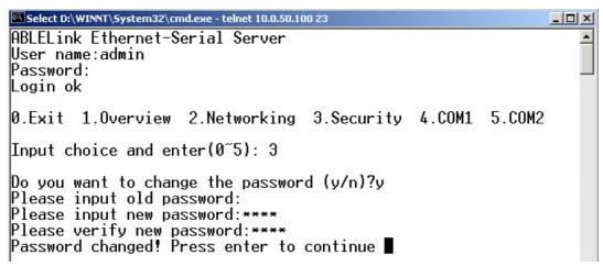
Fig. 13. changing password using Telnet
