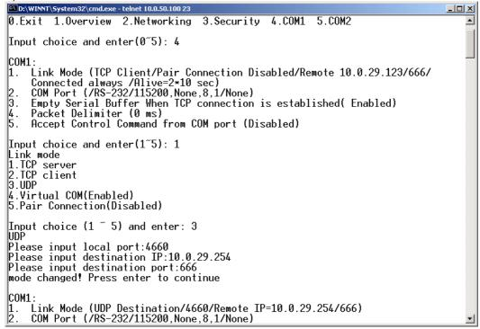
Fig. 17. Link Mode-UDP client setup
