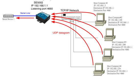
Fig. 32. Data Transmission in a UDP Slave(server) Mode
