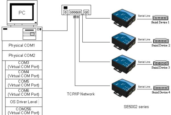
Fig. 35. Virtual Com connection diagram
