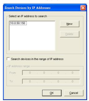
Here user may have two options: Select an IP address to search or Search device in the range of IP address.
