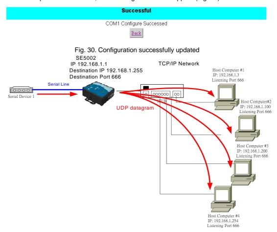
Fig. 31. Data Transmission in a UDP Master(Client) Mode
