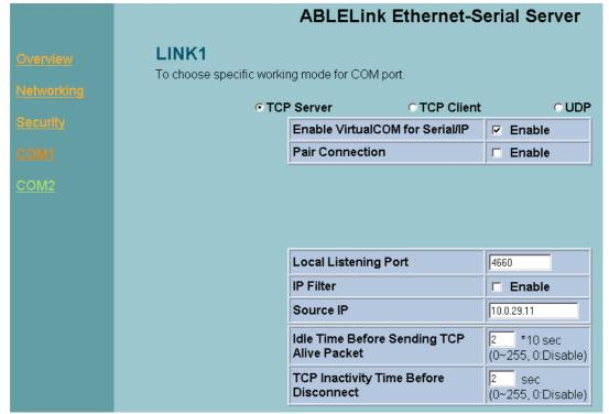
Fig. 36. Enabling Virtual COM port
