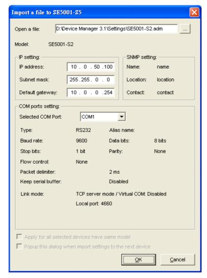
The user can also select several devices at one time, and lead the parameter information of a standard parameter file into all the selected devices by selecting **Apply for all selected devices have same model**.
