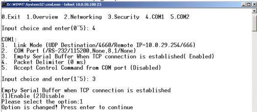
Fig. 19. Com port-Enabling serial data buffer
