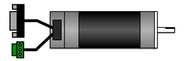
The **MOT-400** is an **180W** brushless DC servo motor. It includes an attached 1000 line encoder that provides position feedback to the drivers. Rated current for the motor is **6.7A**. This motor is flange mounted and compatible with NEMA23 standard sizing. The **MOT-400** has a shaft size of **Ø8.0** mm in diameter with a flat.
