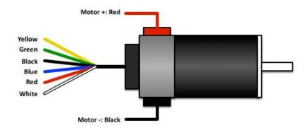
The **MOT-270** is a **50W** permanent magnet DC brush servo motor. It includes an attached 1000 line encoder that provides position feedback to the drivers. Rated current for the motor is **1.79A**.
