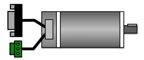
The MOT-455 is a 400W brushless AC servo motor. It includes an attached 2500 line encoder that provides position feedback to the drivers. Rated current for the motor is 8.4A. The MOT-455 has a shaft size of Ø14 mm in diameter with a keyway.
