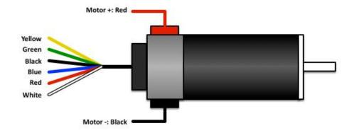
The **MOT-280** is an **80W** permanent magnet DC brush servo motor. It includes an attached 1000 line encoder that provides position feedback to the drivers. Rated current for the motor is **2.95A**.
