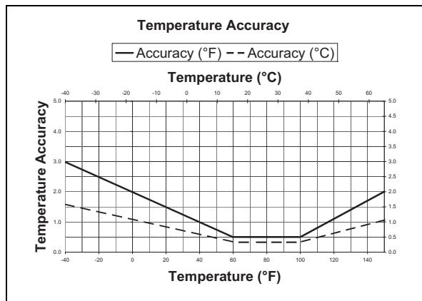
Figure 2. Temperature Accuracy
