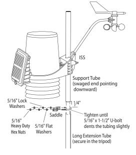
the use of a torque wrench with 25 lb-ft of pressure to fasten the hex nuts. The support tube should be crimped on the extension tube securely to prevent any rocking or rotating.
