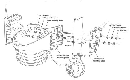
Option 1: Installing ISS and Anemometer Together
