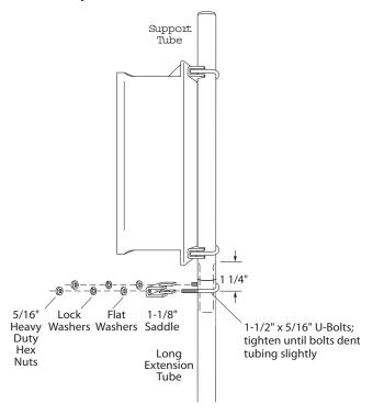
5. We recommend the use of a torque wrench with 25 lb-ft of pressure to fasten the hex nuts.
