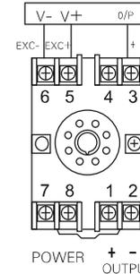
● 4 wire Transmitter or Load cell
