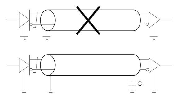
When the shield is connected to ground at both ends, also high frequency interference is avoided. Circulating currents are avoided by a capacitor C in series with one of the ground terminals.
