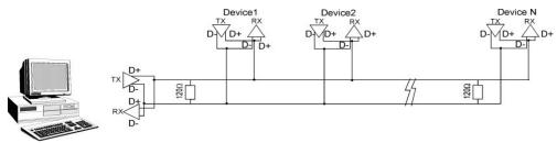
RS-485 interface with plug in board.
