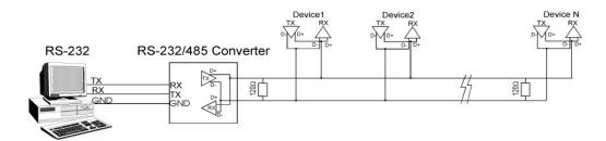
RS-485 interface with seperate converter.
