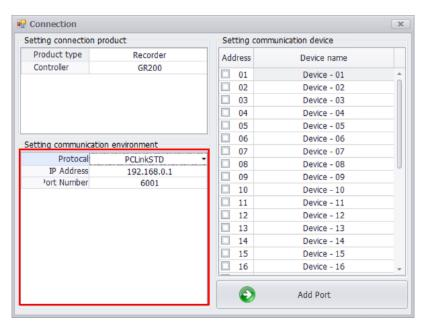
After setting the communication, you can change it in the system screen of the main menu, and you can change the connected equipment too.
