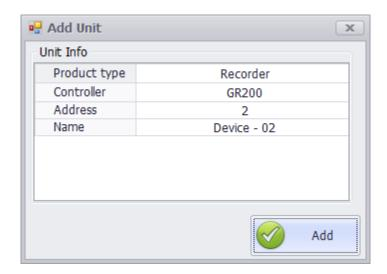
From the add unit window, you can set the product type, product name, device number and unit name. After finishing all the settings, by selecting the add button you can add the unit to the port.
