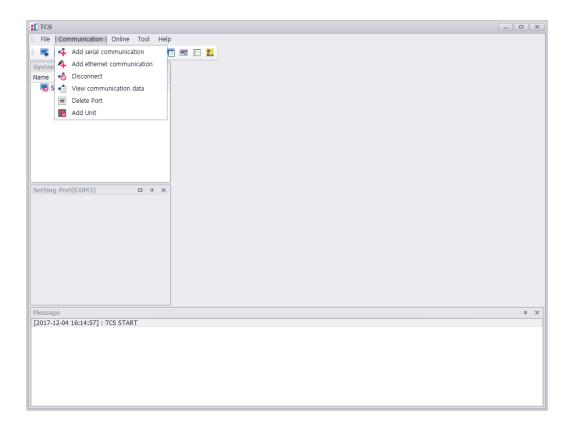
There are two types of communication to add: serial and Ethernet.
