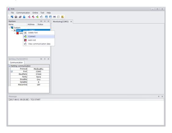
During the first communication, the basic monitoring screen of the equipment is shown automatically.
