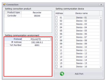
③ " Communication " → "Connect / Disconnect" : connect / remove the selected communication port.
