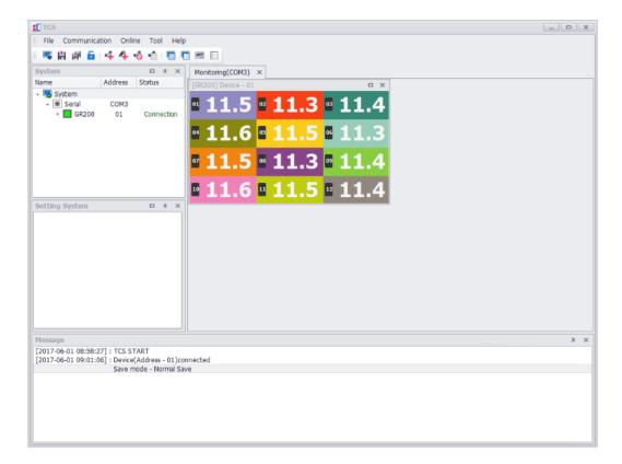
2 " Online "  $\rightarrow$  "TEXT Monitoring : the text-monitoring screen appears ( all equipment monitoring, list view )"
