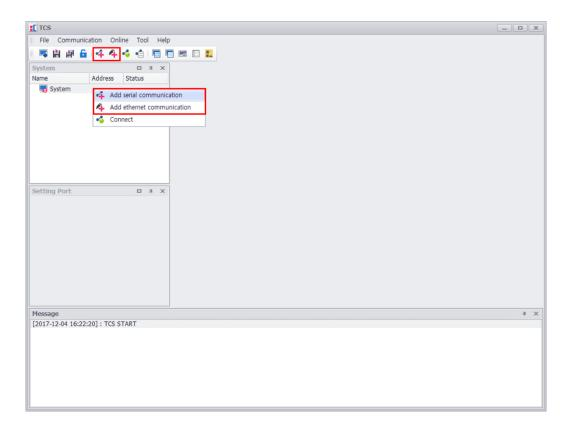
From the communication add window, after setting the communication port and equipment settings, connect the communication.
