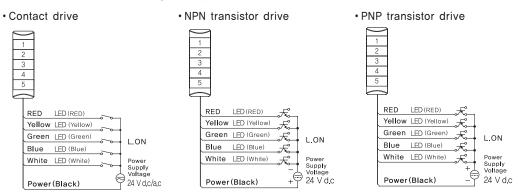
■ WMS-F (Continuous light, Flashing light, Buzzer)
