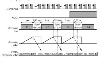
■ Setting rps, 0.1 rpm, 0.1 Hz operation mode
