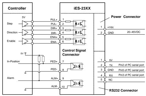
Connect iES-23XX to controller of differential output
