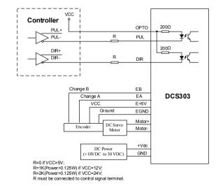
Figure 7: Typical connection (Differential control signal)
