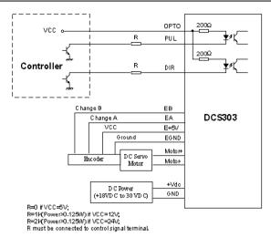
Figure 6: Typical connection (Open-collector control signal.)
