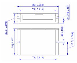
Figure 1: Mechanical specifications
