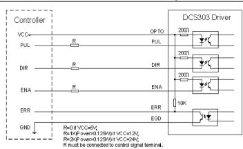
Figure 2: Connections to open-collector control signal (common-anode)
