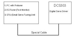
Figure 5: RS232 interface connection
