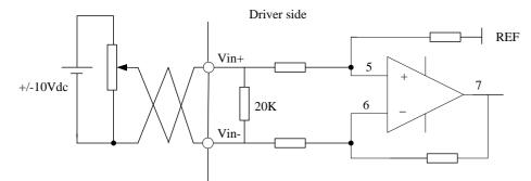
Figure 3-7 Analog Input Interface
