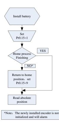
1) Firstly, select the motor with multi-turns absolute encoder which includes battery, and confirm if the drive version supports the function about multi-turns absolute encoder;
