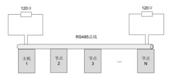
The correct connection of terminal resistance is shown in the above figure, a 120 ohm terminal resistance need to connect in the head end and the end of the communication bus.
