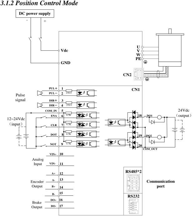
Figure 3-1 Position Mode Wiring
