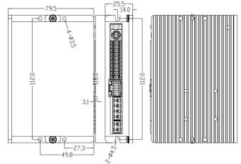
Figure 2.1(A) installation method of drive ELD2-RS7005/ ELD2-RS7010
