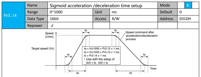
Set S-curve time for acceleration/deceleration process when the speed command is applied. According to Pr3.12 Acceleration time setup and Pr3.13 Deceleration time setup, set up sigmoid time with time width centering the inflection point of acceleration/deceleration.
