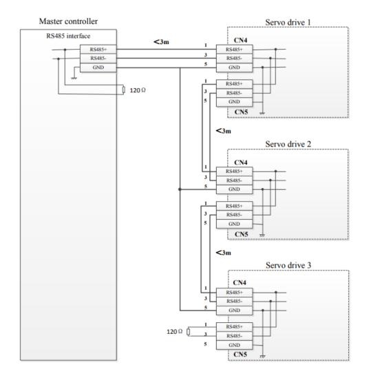
Figure: Multi-drive network connection
