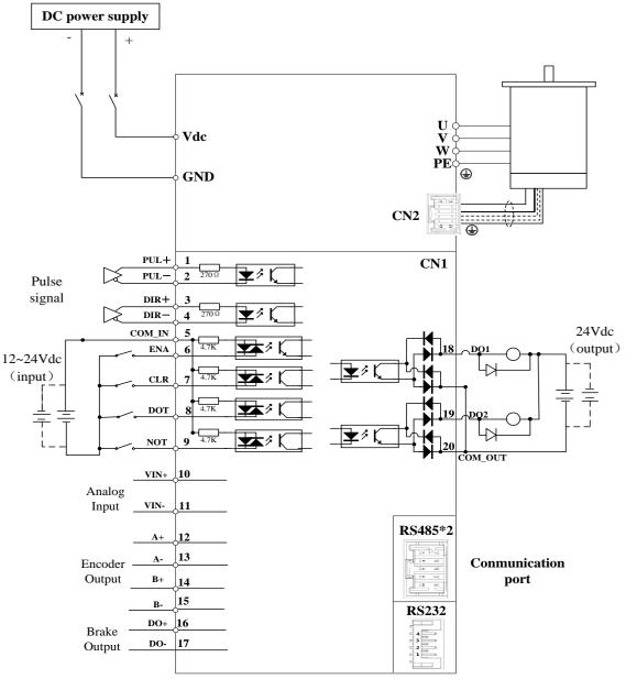
Figure 6-2 Position Mode Wiring
