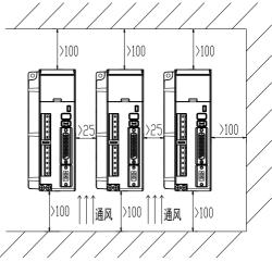
Figure 2.3 Installation Space for several Drives
