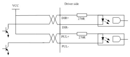
Figure 3-5 Pulse Input Interface Single Terminal Drive Mode
