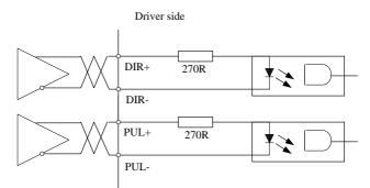
Figure 3-4 Pulse Input Interface Differential Drive Mode
