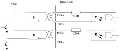
Figure 6-1 CN1 and CN2 Signal Wiring in Position Control Mode
