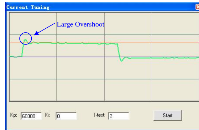
Figure 28: Response with High Kp of current-loop (Kp = 60000)
