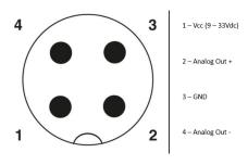
Figure 4 – Electrical connections
