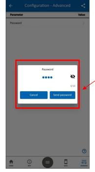
By clicking on the **Password** parameter, you can enter a password that will prevent changes to the device's settings.
