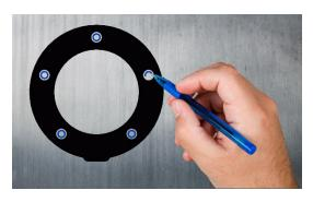
Figure 7 - Marking the gasket
