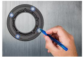
Figure 8 - Marking the adapter (accessory)
