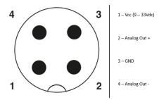
Figure 4 - Electrical connections
