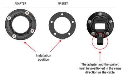
Figure 11 - Installation position
