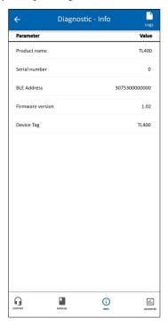
The **Info** section of the **Diagnostics** screen presents information such as serial number, firmware version, BLE address and device tag, which can be set in the **Configuration** section.
