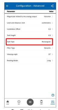
Figure 23 - Volume advanced configurations
