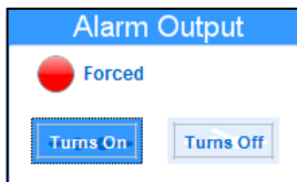
Figure 22 – Alarm output with forcing on status
