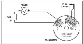
Figure 05 – Transmitter electrical connections – Pt100
