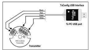
Figure 01 – TxConfig USB Interface connections
