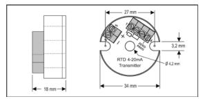
Figure 04 - Transmitter dimensions
