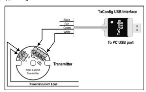
Figure 02 – TxConfig Interface connections – Loop powered
