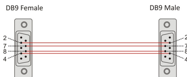
Fig. 26 – Building an extension cable
