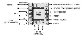
Figure 6 - Electrical connections of NC400-6
