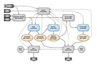
Figure 1 - Diagram with features and resoucers of NC400-6
