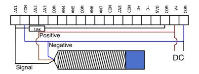
Figure 5 - Wiring a PNP-type sensor
