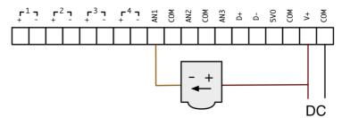
Figure 7 - Wiring a 4-20mA, loop-powered sensor
