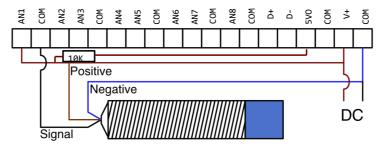
Figure 4 - Wiring an NPN-type sensor
