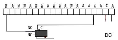
Figure 3 - Wiring a dry contact switch
