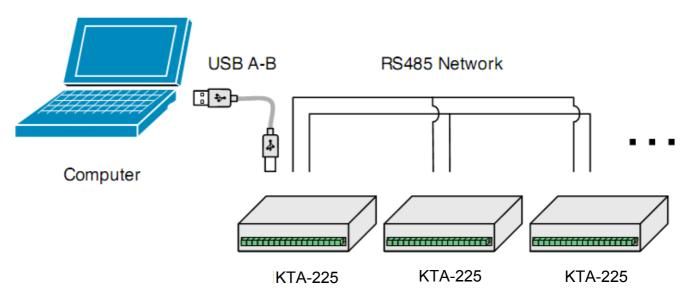
Figure 1 - Connecting multiple controllers with a RS-485 network
