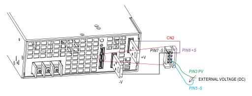
◎ Connecting an external DC source between PV & -S on CN2, and +S & +V, -S & -V also need to be connected as exhibited above.
