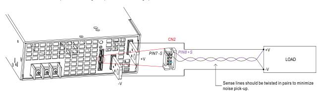
% Caution: The power supply, by factory default(also the assumption for other sections), is shipped with, -S & -V on CN2, as well as +S & +V, shorted by connector. When activating the Remote Sense, the +S signal should be connected to the positive terminal of the load whereas -S signal to the negative terminal.
