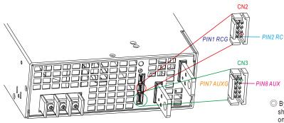
◎ By factory default, PV(PIN3) and PS(PIN4) on CN2 are shorted by connector; likewise, OLP(PIN9) and OL-SD(PIN10) on CN3 are shorted when shipped.
