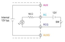
Example 3.2(B): Using internal 12V auxiliary output
