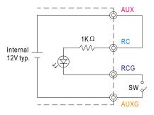
Example 3.2(C): Using internal 12V auxiliary output
