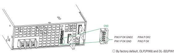
© By factory default, *OLP(PIN9)* and *OL-SD(PIN10)* on CN3 are shorted by connector when shipped.
