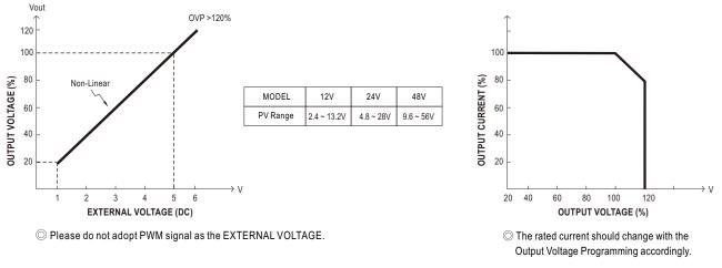
※ Caution: (1)By factory default, the Output Voltage Programming is not activated, and PV(PIN3) and PS(PIN4) of CN2 are shorted by connector. Whenever this function is not needed to activate, as assumed in other sections' diagrams, please keep PV(PIN3) and PS(PIN4) of CN2 shorted; otherwise, the power supply will have no output.
