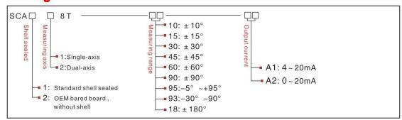
E.g: SCA118T-10-A1: single-axis/standard/±10° Measuring range /4mA-20mA output current
