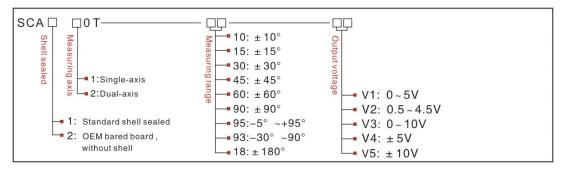
E.g: SCA110T-10-v1: single axis/standard/±10°Measuring range/0V-5V output voltage
