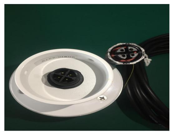
The communication cable is 4 cores for RS485 output , and the connection method is as follows:
