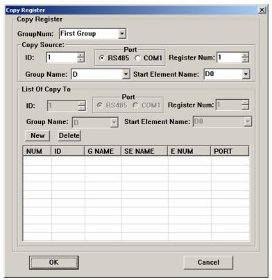
Users can set 3 groups of relationships about registers transferring. Every communication scanning cycle, OP10 will check the synchronization between source PLC and those of destination PLC once. If source PLC has communication errors, OP10 won't update the registers of destination PLC. Every corresponding relationship contains one group of source addresses, 5 groups of destination addresses and can transfer 16 seriate word registers (not support double words register transfer) at most.
