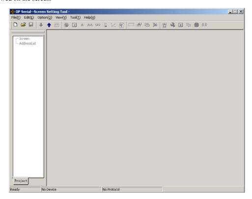
The screen-editing region is on the center of the editor. There is a grid of white dots in the display region. The distance between every two rows and two columns is 16 points. The whole region is a matrix of 192\*64 points. The user can refer to the dots nearby to align the components when laying or moving them. When necessary, change X and Y positions of the components to locate them in arbitrary positions.
