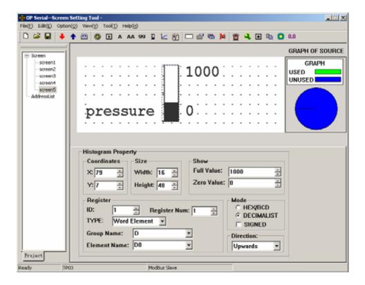
The bar graph demands the data in D0.When the bar is full, it means the data is 1000 in D0.When the bar shows the scale of 500, it means the data is 500 in D0.
