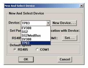
Select the proper PLC type. Then click "Set" button down beside the port name to set communication parameter.
