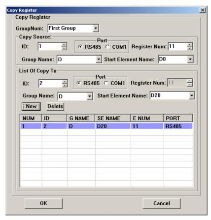
It doesn't matter that source PLC and destination PLC are not on the same bus. OP10 can use download port to communicate with source PLC, then send the data of registers to the destination PLC through 485 bus. Users only need to choose the communication port in the dialogue box simply.
