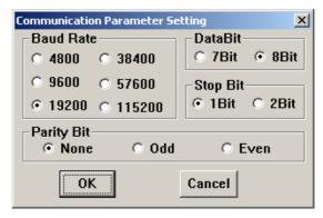
Select the proper baud rate, data bits, stop bits, parity and communication port in the dialog box. OP10 supports the function that two communication ports can connect with different PLCs and transducers using different communication formats.
