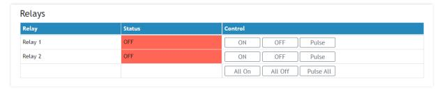
This section displays the current state of the relays. Each relay can be activated either remotely or locally based on the status of a monitored parameter. For relays activated locally, a text description of the controlling parameter is shown instead of control buttons.
