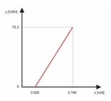
The sensor outputs raw voltage values, but our goal is to convert these into corresponding relative humidity (RH) values. To achieve this, we use a multiplier and an offset. These parameters enable us to calculate the relative humidity for any voltage within the sensor's operational range.
