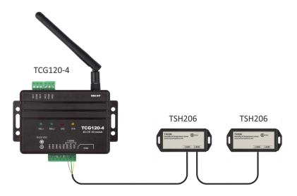
"Star" topology may be used as a last resort, but only for connecting up to four sensors with a total cable length not exceeding 10 meters:
