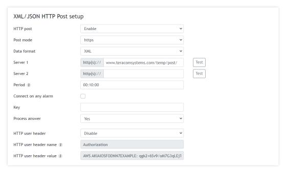
The HTTP POST method is used for the periodic upload of XML/JSON files to a server via HTTP/HTTPS requests (POST method). These files contain the current status of all monitored parameters along with additional system information. The format of the file (XML or JSON) can be selected from a drop-down menu.
