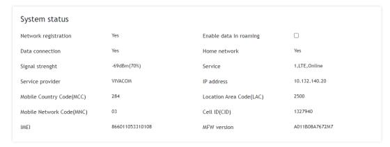
The only configurable setting in this section is the "Data in roaming" checkbox. By default, this option is disabled to prevent additional charges for data usage while roaming.
