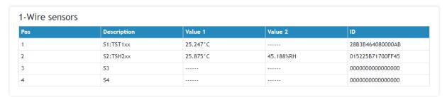
The TCG120-4 module supports up to four sensors. All detected 1-Wire sensors are displayed in the "1-Wire sensors" section. These sensors need to be configured in the "1-Wire sensors setup" section, accessible via the Setup -> Sensors page.
