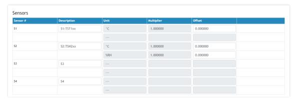
For each sensor, a description of up to 15 characters can be set. These descriptions will appear on the monitoring page, conditions page, in XML/JSON data, as well as in SMS and email alerts.
