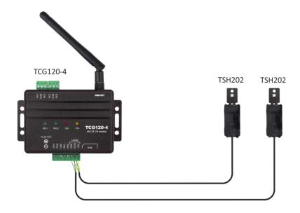
It is strongly recommended to use only UTP/FTP cables for the 1-Wire interface and to keep the total cable length within 30 meters. While functionality has been observed at longer distances, error-free operation cannot be guaranteed beyond the specified limit.
