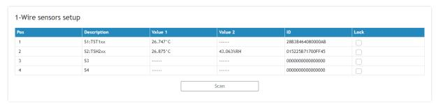
Detection of connected 1-Wire sensors occurs automatically at power-on or can be triggered manually by pressing the "Scan" button. All detected sensors are displayed in ascending order according to their unique ID numbers.
