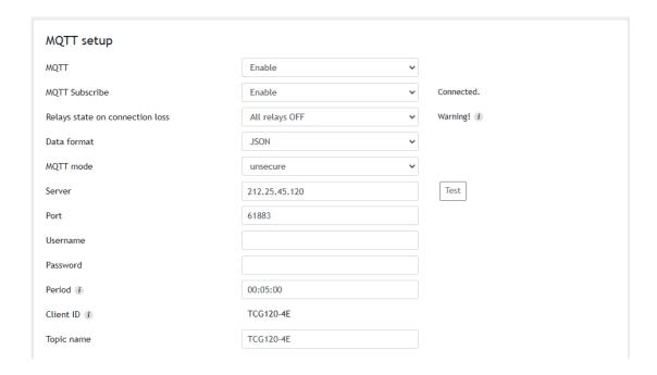
Messages can be sent to the MQTT broker in JSON or plain text format, with an option for an encrypted (TLS) or unencrypted connection. In case of a connection loss with the MQTT
