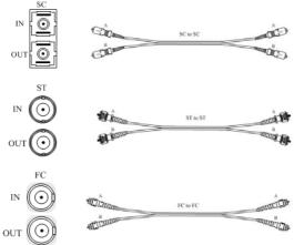
**NOTE:** SC, ST or FC, for optic fiber interface, SM is look the same to MM for form. For example,Model277 SM/A /SC, the optic fiber interface(SC) is look the same to Model277 MM/A/SC.
