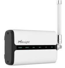
UG65 is a robust 8-channel indoor LoRaWAN<sup>®</sup> hotspot, which is compatible with Helium LongFi technology. Adopting SX1302 LoRa chip, high-performance quad-core CPU and secure crypto chip, UG65 provides high-efficiency and reliable connection. UG65 has line of sight up to 15 km and can cover about 2 km in urbanized environment, which can cover larger areas and provide connectivity to more than 2000 nodes.
