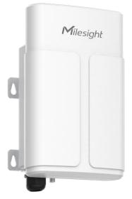
UG67 is a robust 8-channel outdoor LoRaWAN® hotspot, which is compatible with Helium LongFi technology. Adopting SX1302 LoRa chip, high-performance quad-core CPU and secure crypto chip, UG67 provides high-efficiency and reliable connection. UG67 has line of sight up to 15 km and can cover about 2 km in urbanized environment, which can cover larger areas and provide connectivity to more than 2000 nodes.
