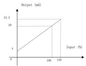
$4 \text{mA}{\sim}20 \text{mA}$  Input-Output characteristic curve
